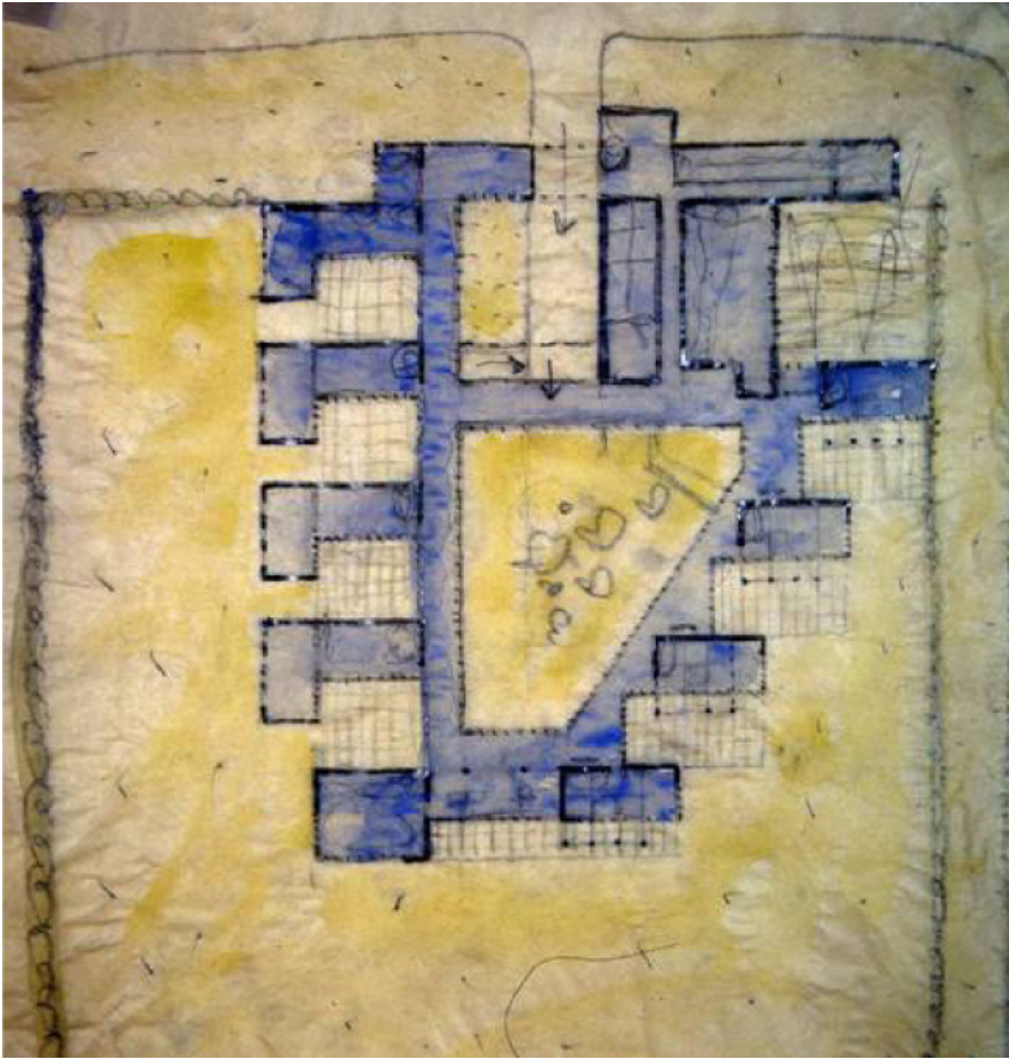
Fig. 14 The wish to provide each unit with an outside area and to distinguish the younger children's units from those of the seniors results in a different way of linking the groups. As in 13, the younger children's units are shifted with respect to one another and laid out along a diagonal street.
