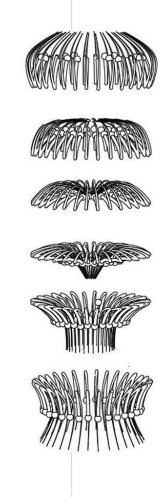
The goal of this project is to harvest the excess water and turn it into energy that will power the entire city, while also providing a community gathering space for the inhabitants of the islands as they adapt to their new reality. The water flows into the centre of the structure, where it is guided to fall down towards the turbine located below the dome.
